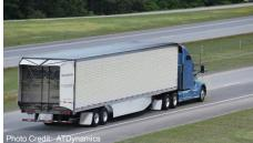
Certified to deliver 6.6% fuel efficiency gains at 65 mph based on SAE Type II testing validated by the U.S. EPA, sufficient for standalone pe it testing validated by the U.S. EPA, sufficient for impliance with 2010 CARB regulations for trailer aer rempt from U.S. DOT length restrictions.
